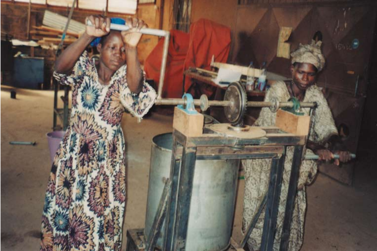
Participatory technology development increases the potential for local processing. Here the example of the locally developed shea butter churn (Photo by Jean-Marc Tendon).
